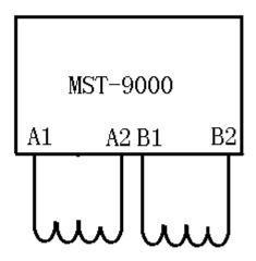
MST-9000 driver 6-line Step Motor connection method:
