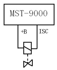
MST-9000 driver pressure control valve connection method:
