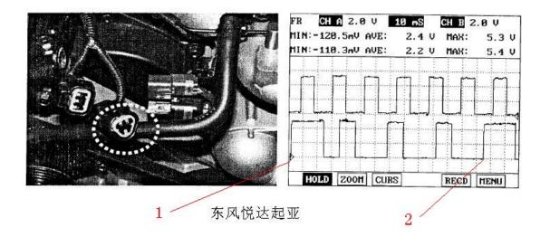
Attention: the phase diagram of crankshaft signal and camshaft must be a whole working cycle WAVEFORM, as the above showing:
