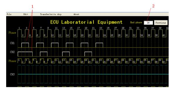
Notes: CH1/CH2 is Hall sensor signal output, CH3\CH4\CH5 is magneto electric sensor signal output
